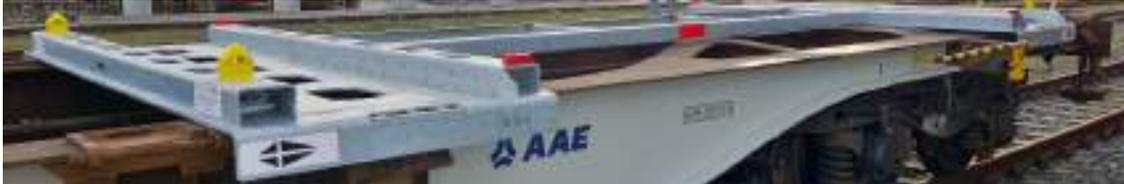
Figure 18 – Wagon adaptor with “cross hairs sign” for positioning
