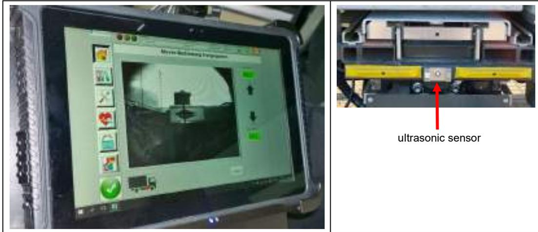
Figure 13 – The screen in the cab and one of the ultrasonic sensors
