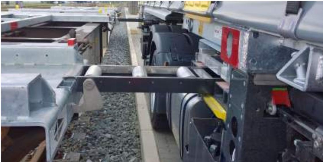
Figure 15 – The contact bridge between ContainerMover and Wagon Adaptor
