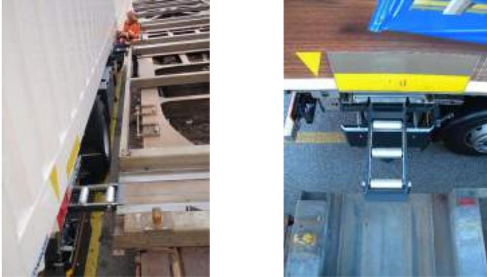
Figure 5 – The two “contact bridges” between truck and railway wagon
