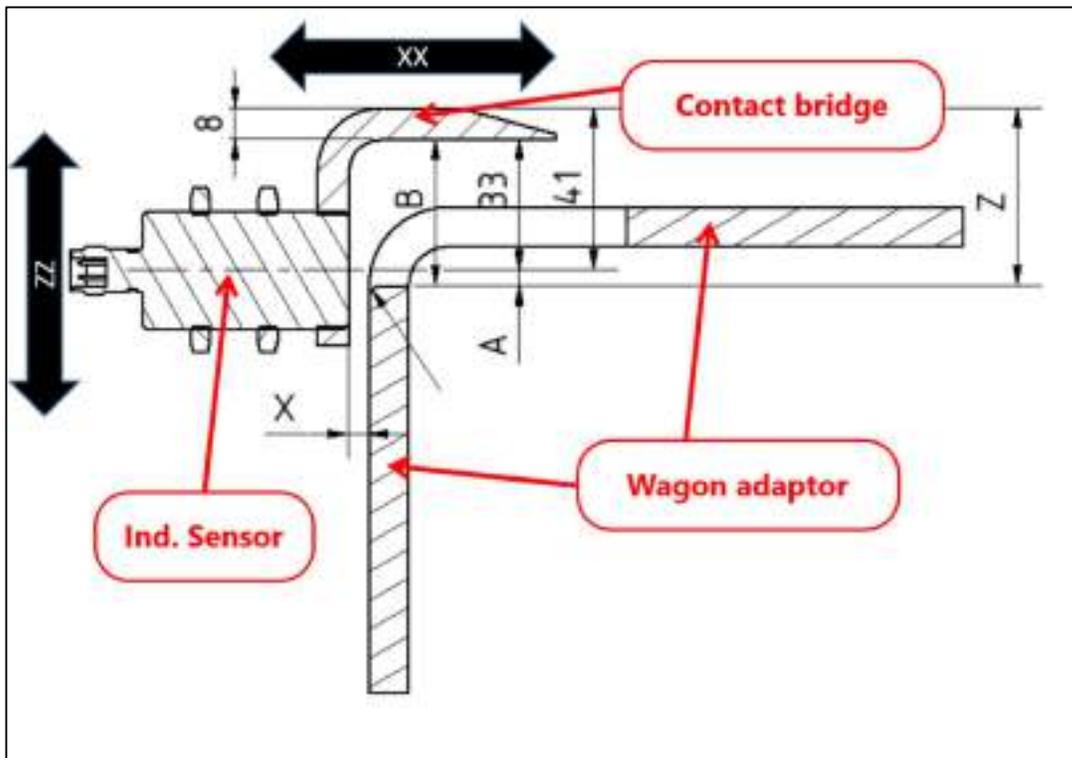
Figure 35 – drawing of tip of the contact bridge and wagon adaptor sector
