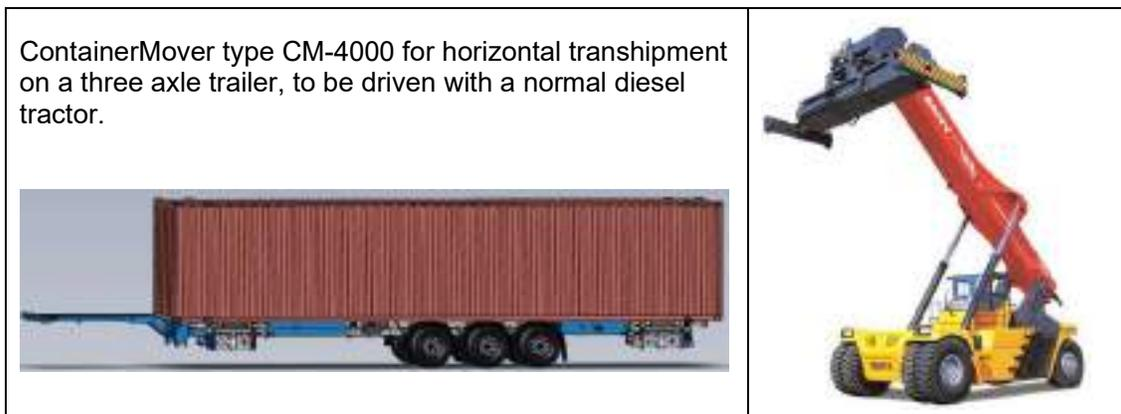
Figure 37 – ContainerMover-4000 and Reach Stacker
