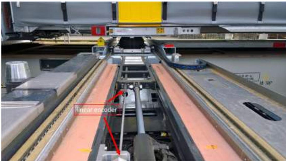
Figure 14 – the linear encoder for measuring the exact distance the contact bridge is ejected.
