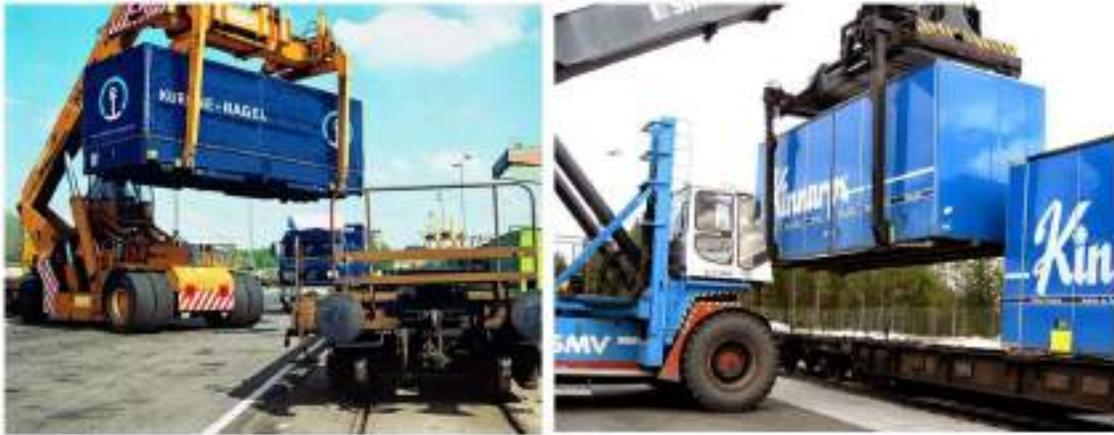
Figure 30 – reach stacker using crappler arms for a swap body
