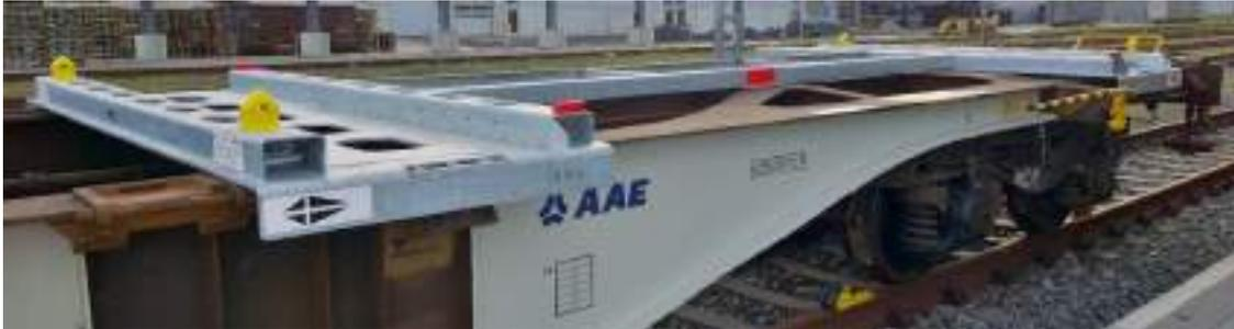
Figure 3 – Wagon adaptor frame on 20' position
