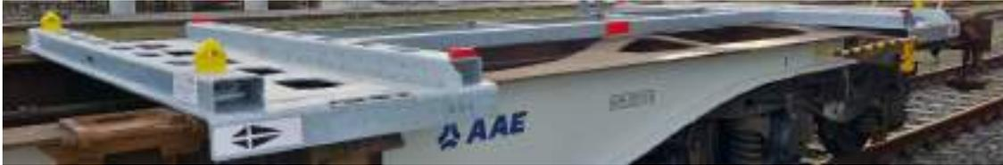
Figure 7 – Wagon adaptor with “cross hairs sign” for positioning
