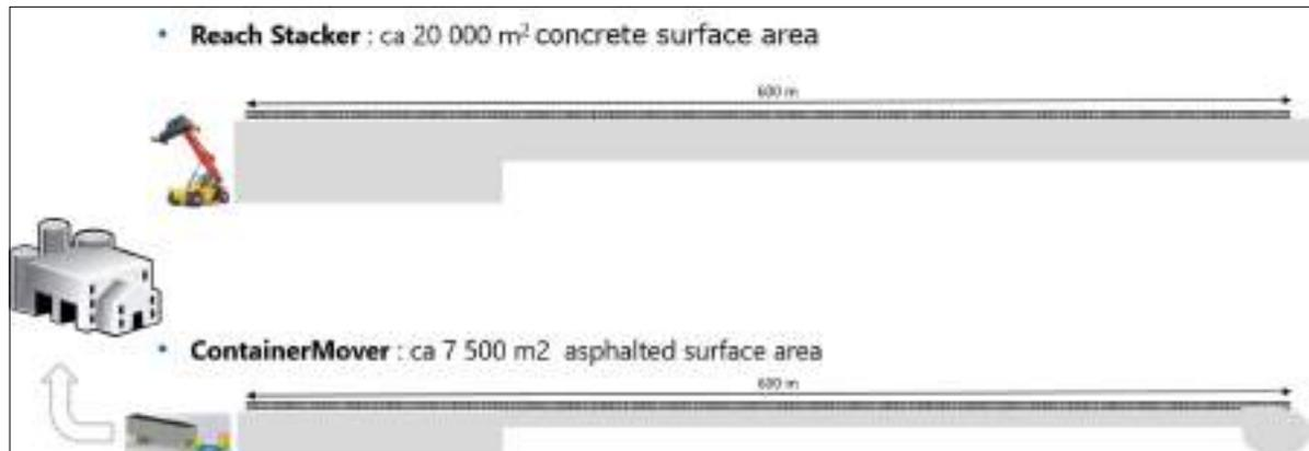
Figure 38 – working surface for a ContainerMover-4000 and for a Reach Stacker
