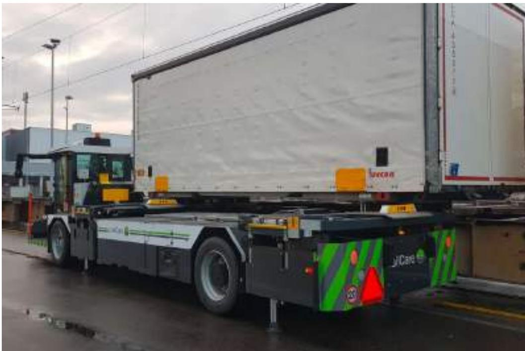
Figure 24 – ContainerMover 3040 (Picture railCare)
