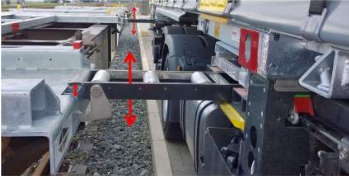
Figure 16 – Adjusting the height of the two “contact bridges”
