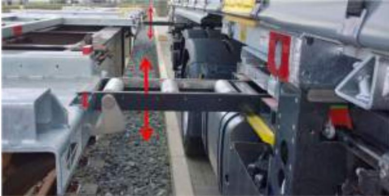
Figure 32 – Adjusting the height of the two “contact bridges”
